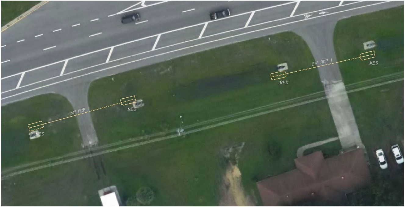
Comparison of existing storm drainage mapping from legacy data supplied by the owner to the current aerial imagery collected for the project.
