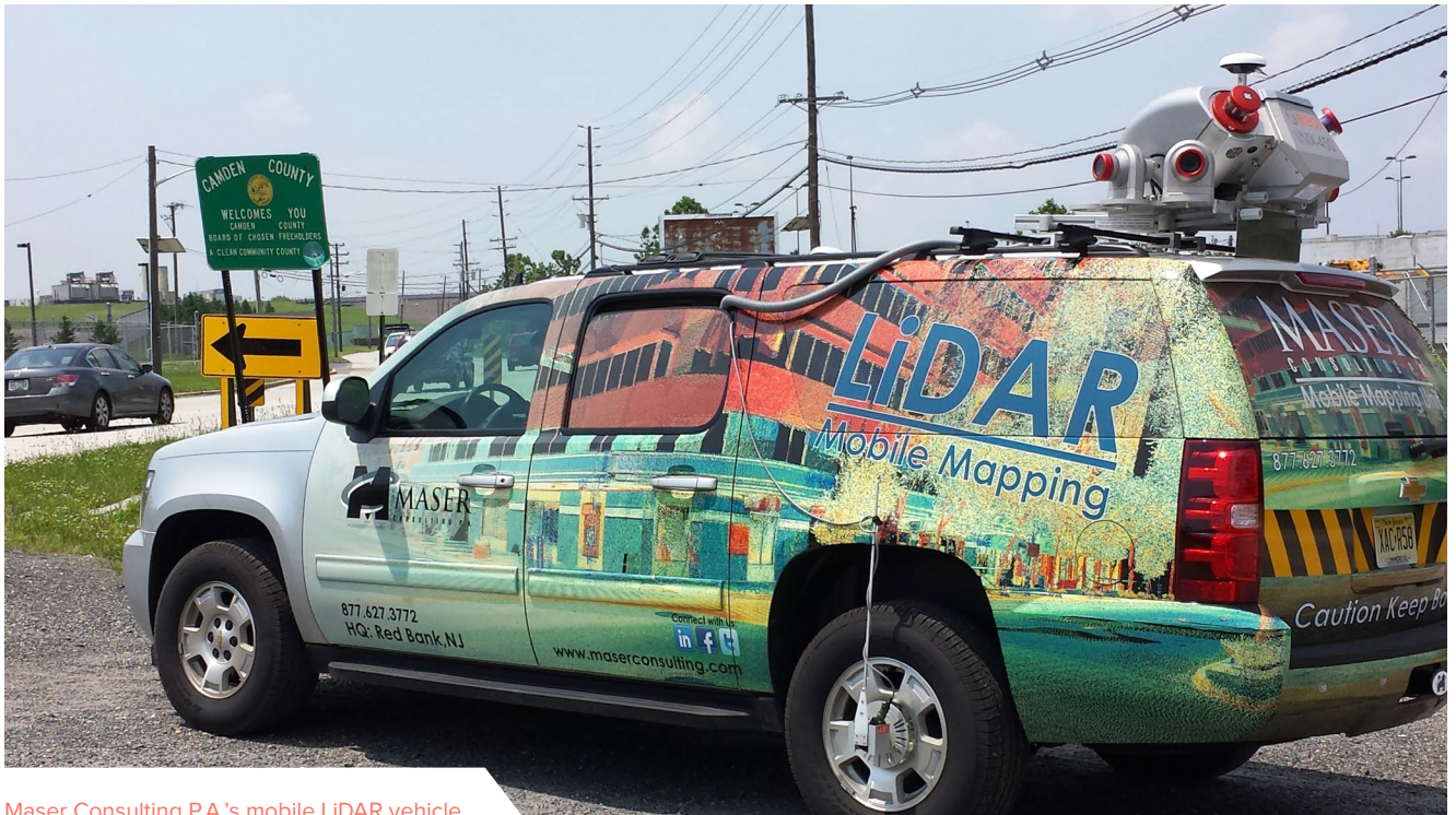
Maser Consulting P.A.'s mobile LiDAR vehicle
