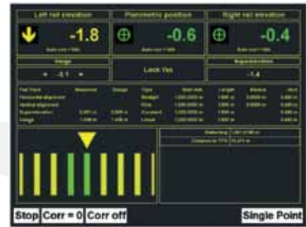
Left: A sample dynamic clearance cross-section in Amberg Rail software. Below left: Three-dimensional Autodesk AutoCAD drawing exchange format files of tunnel wall cross-sections with Metro Transit Authority car-body data overlaid onto laser scan data for the No. 7 subway extension project in New York City. Above: A screen capture of Amberg Slab Track software showing track adjustment criteria. Images courtesy of Maser Consulting
